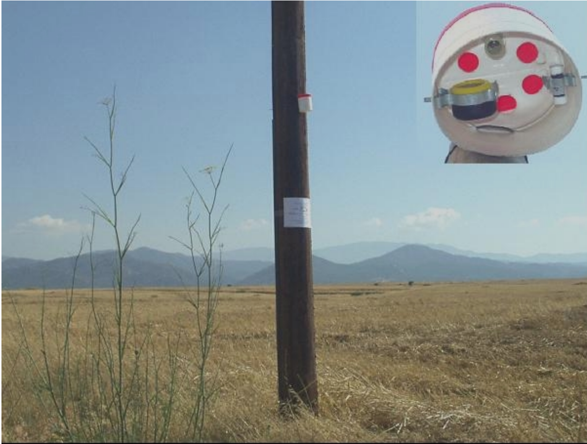
Figure 3.1. Shelter with Diffusive Samplers used in the field
